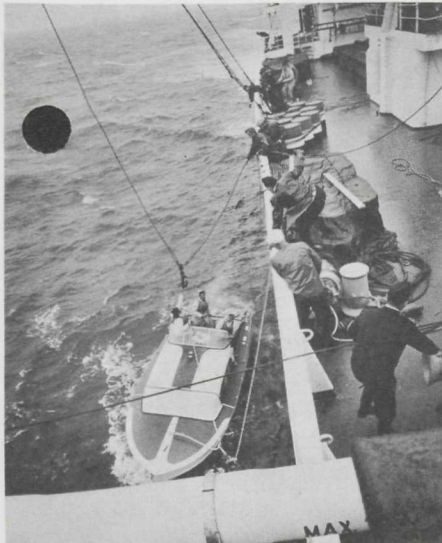
Pick-up at sea: Triangular rope device hauls the Coronet Explorer aboard its escort ship, the Clary Thordén.
