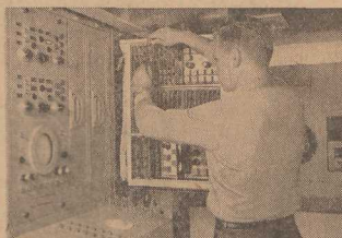
Data Processors, which monitor hundreds of aircraft and store the information for high-speed assignment of defense weapons, comprise one part of an advanced Hughes ground defense system.
