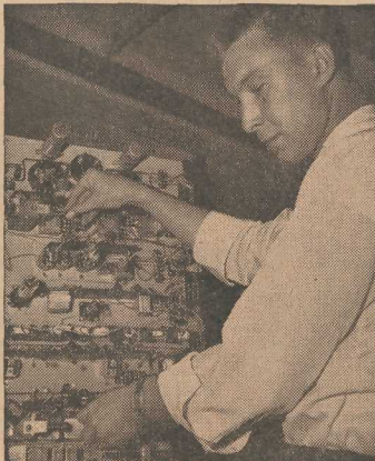
Bob Wilson works on a "breadboard" circuit, studying the electrical properties of a carrier system.
